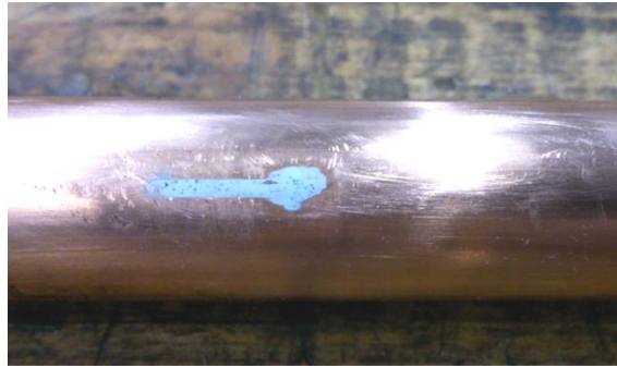
Figure 3-7: An embedded thermocouple.
