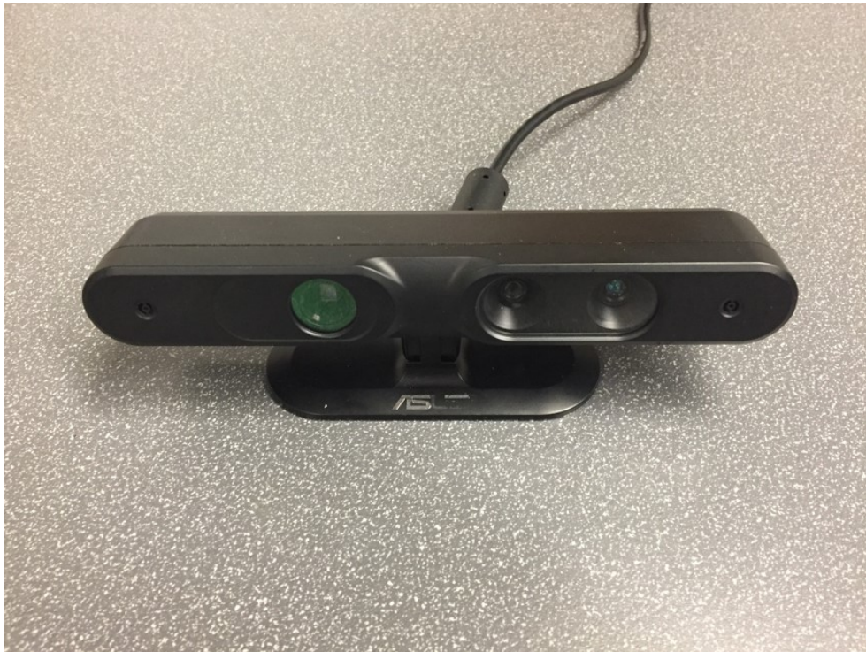
Figure 3: Asus Xtion Vision Sensor
