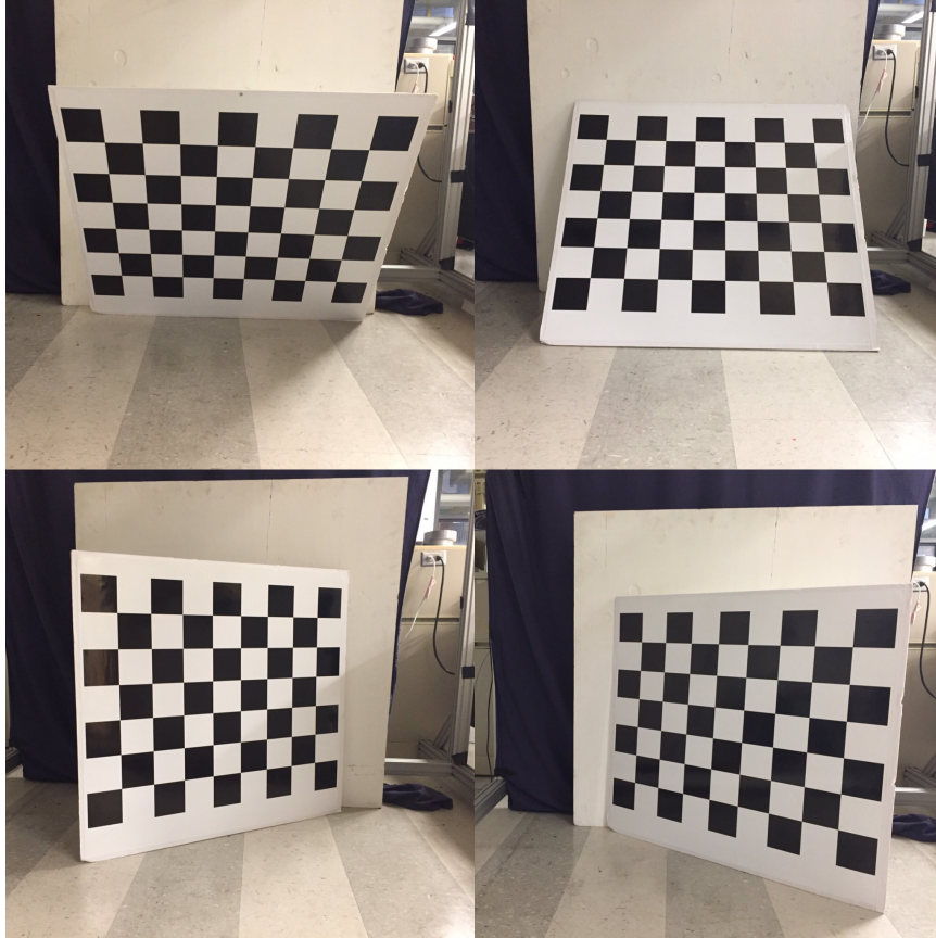
Figure 37: Samples of the Different Orientations Used to Calibrate the Sensor
