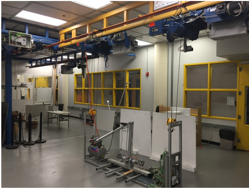
Figure 2: Two-Ton Dual-Hoist Bridge Crane with Robot.
