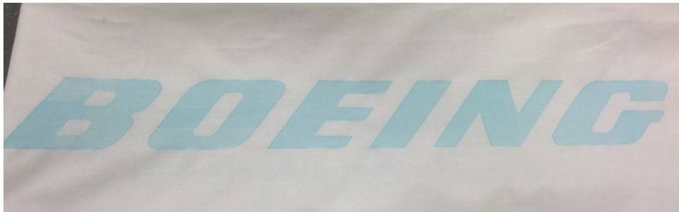
Figure 50: Boeing Logo Painted Using Air Brush End Effector
