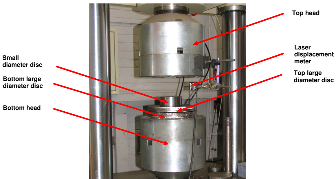
Figure 3-1: Test setup used for the material characterisation of the packing materials
