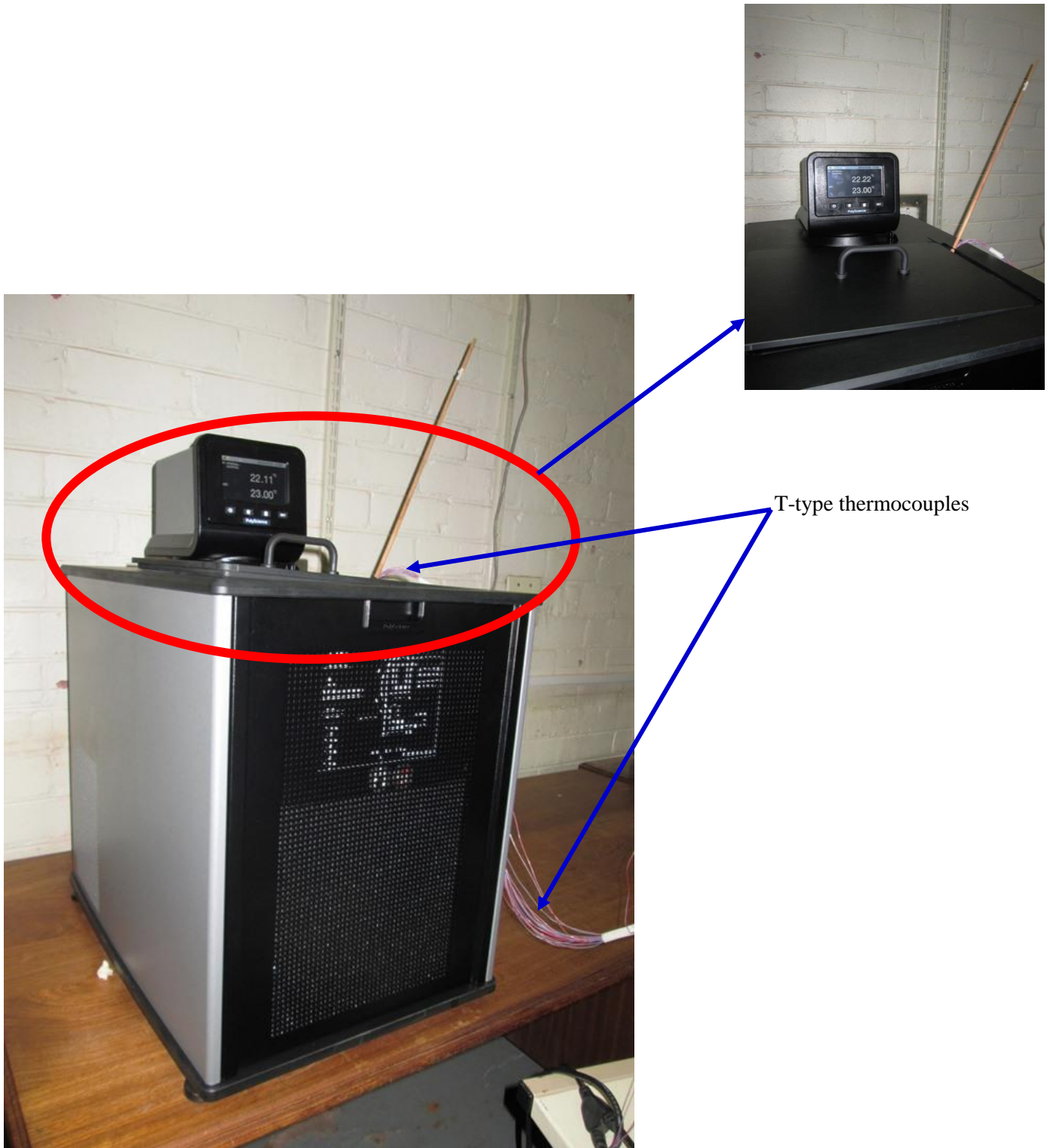
Figure A-2 PolyScience circulating bath (PD20R-30-A12E) used for calibration
