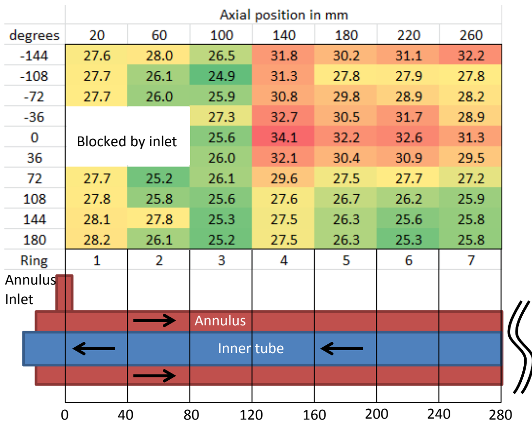
Figure 22 – Temperature distribution at inlet for cooled annulus ( Re \approx 13\ 800 )
