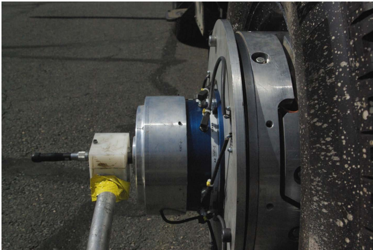
Figure 14: Wheel force transducer mounted on test vehicle
