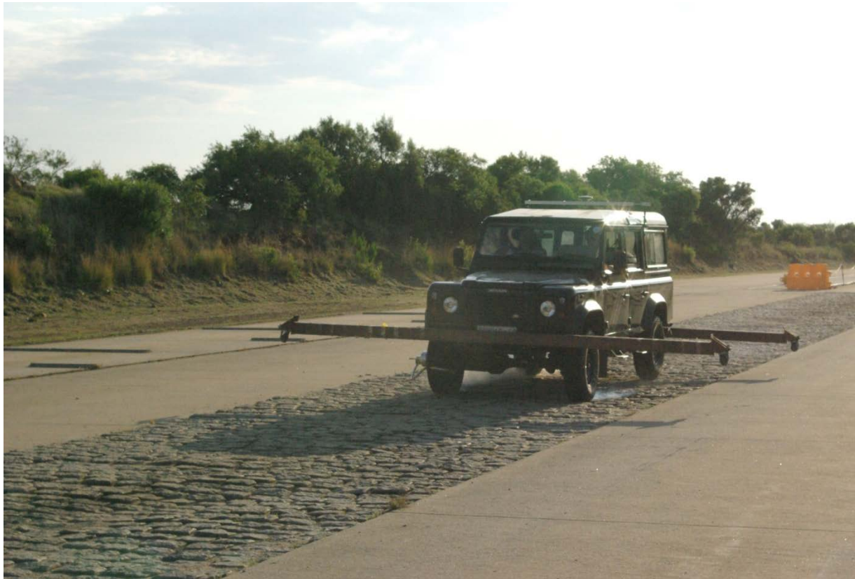
Figure 22: Test vehicle performing brake test on Belgian paving
