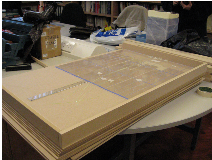
Figure 3.3.2: Scintillator tiles, produced in Russia. The optic fibres inside their grooves are also visible.
