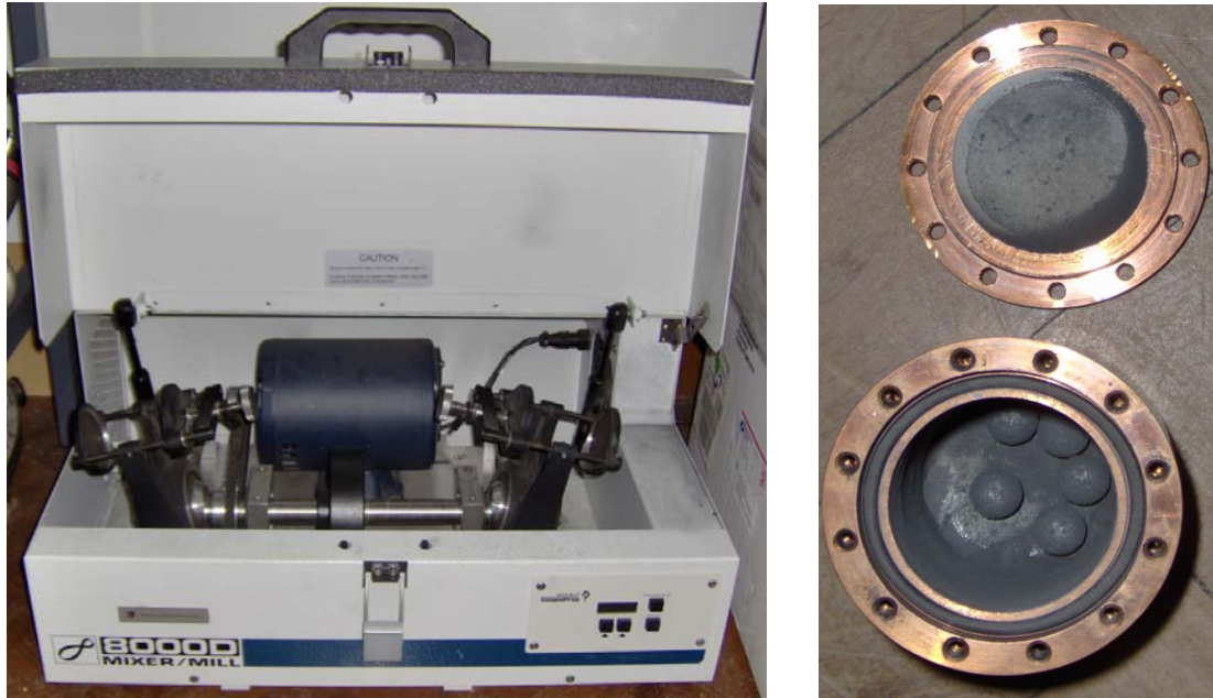
Figure 4.14 (a) SPEX 8000 D mixer/mill in the assembled condition with a copper vial (b) Copper vial set consisting of the vial, lid, o-ring, and balls (10 mm diameter).
