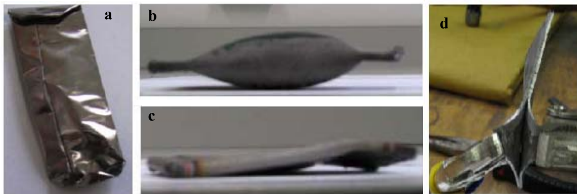
Figure 5.2 Different stages of the billet preparation (a) Powder wrapped in niobium foil; (b) Sealed billet before consolidation; (c) HIP'ed billet; (d) Bulk sample recovery [137].
