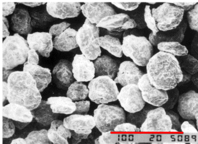
Figure 3.62 Scanning electron micrograph of Nb-Al as-milled powder. The read marker is 100 μm [98].
