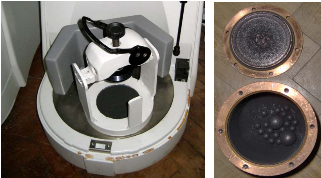
Figure 4.13 (a) Fritsch planetary mono-mill (Pulverisette 6) in the assembled condition; (b) Copper vial set consisting of the vial, lid, o-ring, and balls (20 and 10 mm diameter).
