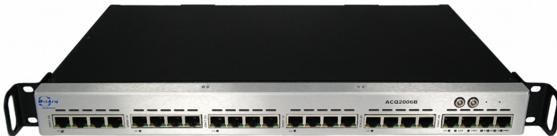
Figure 2.3: Top: the BOLO8 module, showing the 4 RJ-45 connectors to connect to 8 sensors, the long black ELF connector for connection to the ACQ2106 and 8 of the inductors used in the LC filters. The 8 channel module is extremely compact compared with previous analogue generations. Bottom: 6 BOLO8 modules in an ACQ2006 carrier, providing 48 channels in a 1U, 19-inch form factor. Reproduced from [62]
