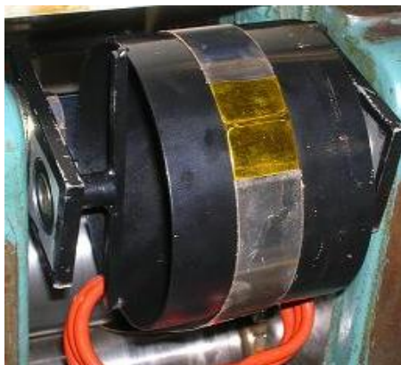
Figure 3-3: Adhesive connection between mold ribbons.
