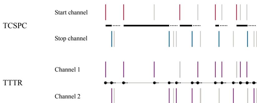
Figure 8.5: Diagrammatic comparison between the two FIFO modes of the coincidence detector hardware: time-correlated single photon counting (TCSPC) and time-tagged time-resolved (TTTR). The first obtains time differences between start (red) and stop (blue) channels; the second, obtains the time-tags of the events (purple) in each of the channels. After registering a time difference or a tag, the dead-time of the counting module prevents other detections from being immediately recorded.
