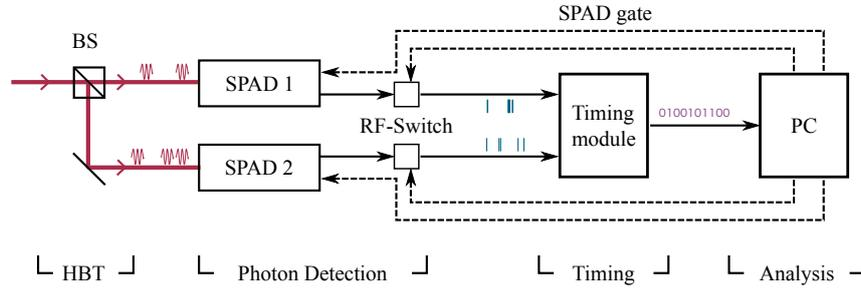
Figure 8.1: Detection system to determine  $g^{(2)}$ . A Hanbury-Brown-Twiss (HBT) interferometer divides the light using a beamsplitter (BS), which is then detected using single-photon avalanche photodiodes (SPADs) and the detections are converted to electronic pulses. The pulses are sent to the timing module. Finally, the data is collected in the computer for later processing.
