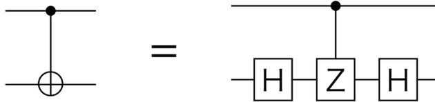
Figure 6.1: A CNOT gate (left) can be implemented by connecting two Hadamard gates to a CZ gate (right).
