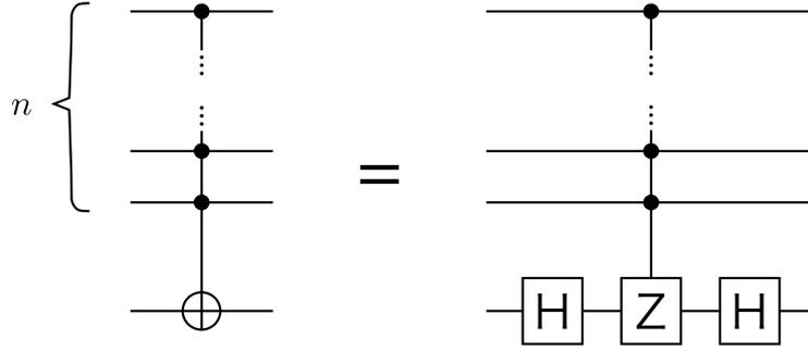
Figure 7.1: A  $C^n Z$  gate (left) implements a Pauli-Z rotation on the target qubit dependent upon  $n$  control qubits. It can be converted into the  $C^n \text{NOT}$  gate using two Hadamard gates (right).
