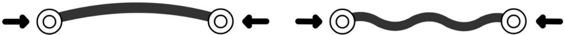
Figure 1-8: Buckling with a vertical restoring force (right) compared to buckling without a restoring force (left).
