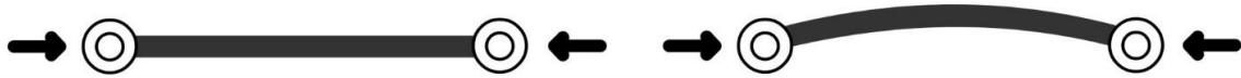
Figure 1-7: Buckling of a slender object under uniaxial compression and hinge boundary conditions. Note that only half a wavelength is covered within the domain.
