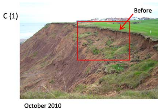
Figure 5.2 A diagram of the reactivated landslide at the upper section of the Upgang cliff at which instruments were installed (A). The extensometer consisted of a cable that was anchored on the main scarp of the landslide and extended up to and past the ground surface recording landslide displacement (B; i.e. VBW1 and S4). The photos show the upper part of the cliff before failure in 2010 (C1) and after failure in 2011 (C2).
