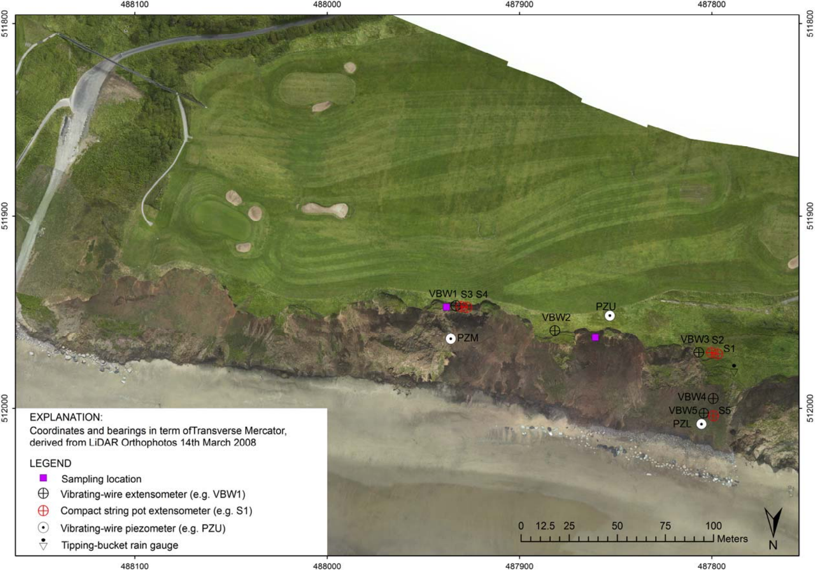
Figure 3.9 Map of the Uppang monitoring instruments including ten extensometers (VBW1, VBW2, VBW3, VBW4, VBW5, S1, S2, S3, S4, and S5); three piezometers (PZU, PZM and PZL) and a rain gauge. Note: VBW – vibrating-wire extensometer; S – compact string pot extensometer.
