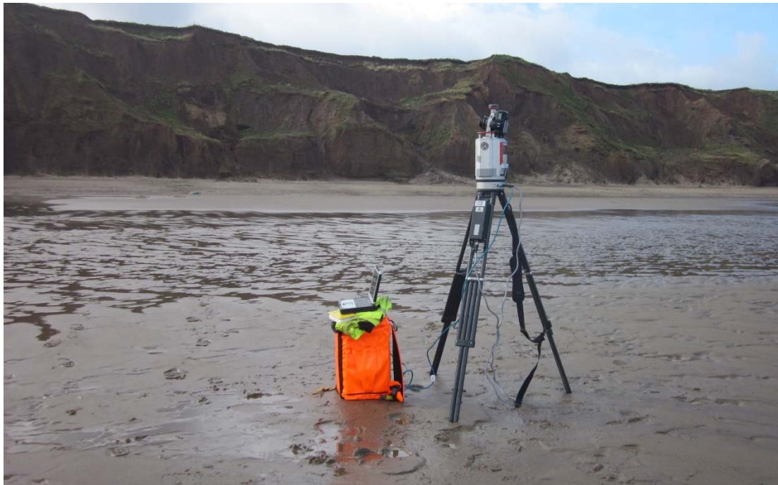
Figure 3.5 Photographs of two devices: a) Trimble GS200 device includes a tripod, a laser scanner, a generator and a computer; b) RIEGL VZ 1000 consists of a tripod, a laser scanner and a computer
