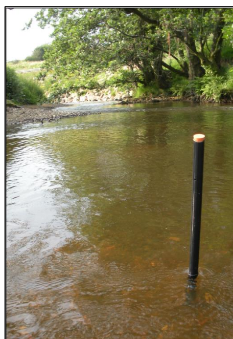
Figure 4.3. Plate of hyporheic sampling well Location: MP8, Danby (Sewage Treatment Works)
