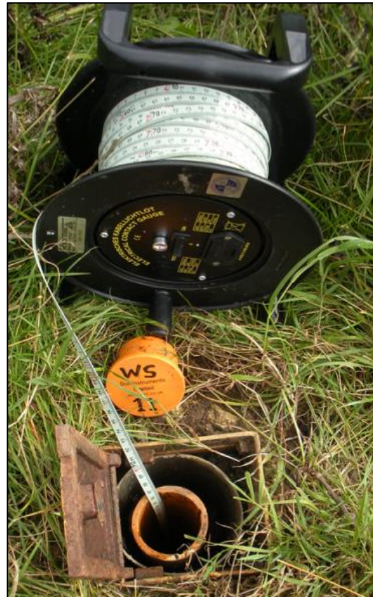
Figure 4.6. Danby Sewage Treatment Works – Borehole and Dip Meter Reading
