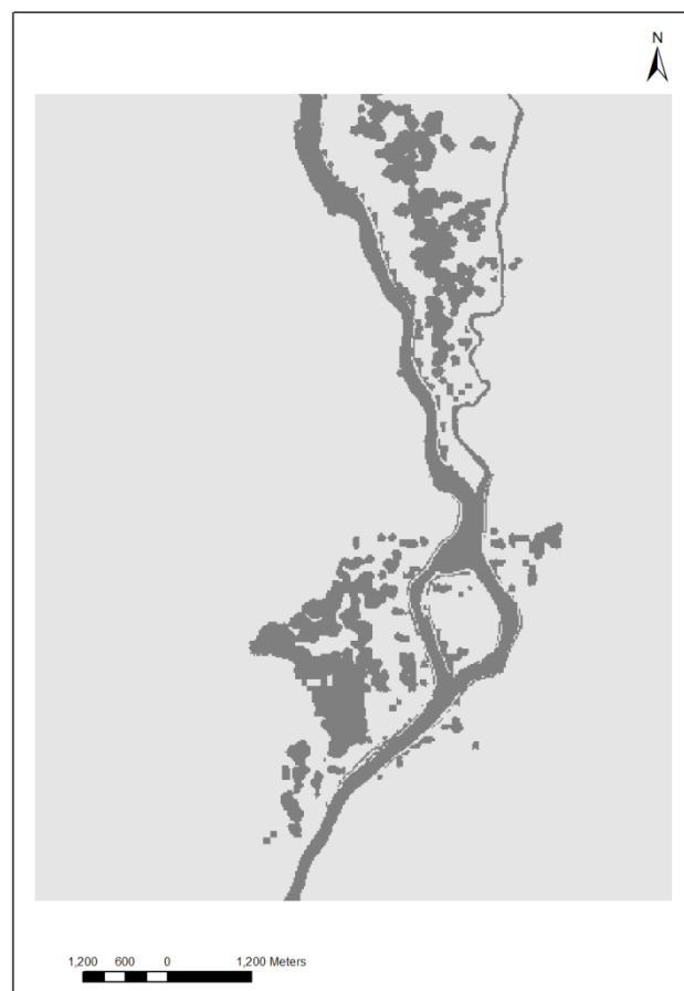
Figure 4.13 Modelled flood extent of the TELEMAC2D using the SRTM DEM at the time step coinciding with the IRS Resourcesat-1 satellite overpass (Figure 4.10 c).
