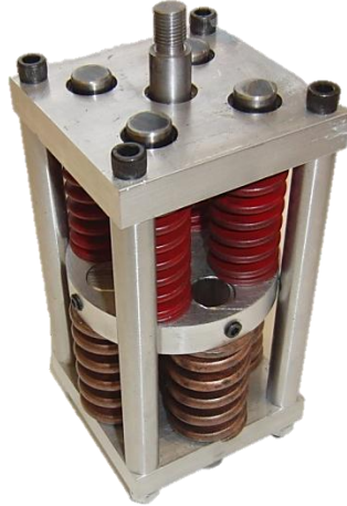
Figure 22. Linear foot spring mechanism having independent stiffness values for plantar flexion and dorsiflexion in the linear domain.
