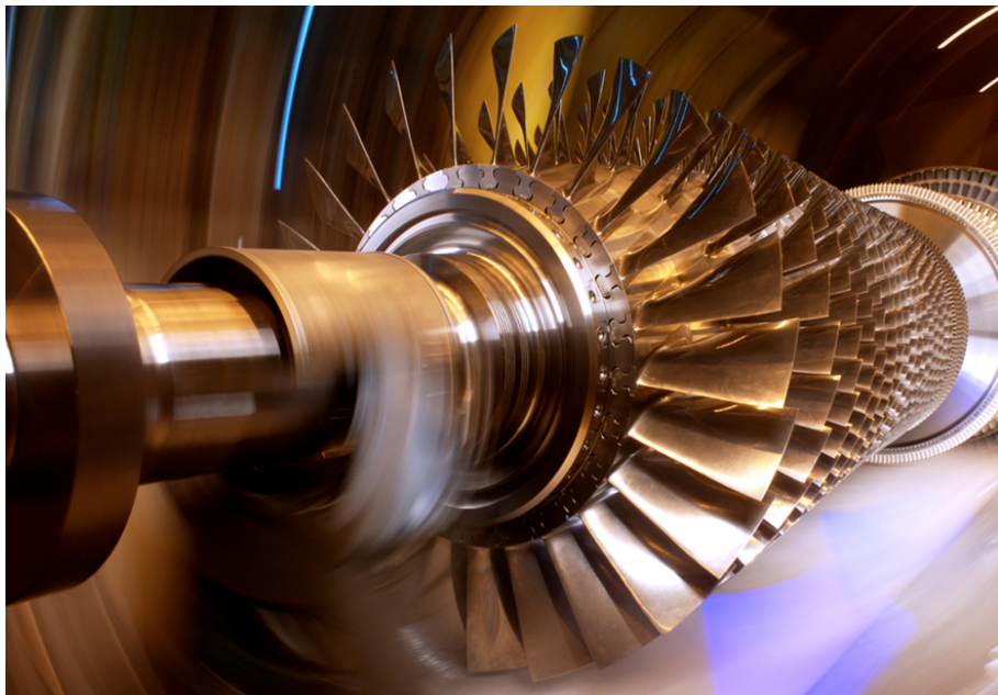
Figure 1.1: A partially constructed land based gas turbine [1]
