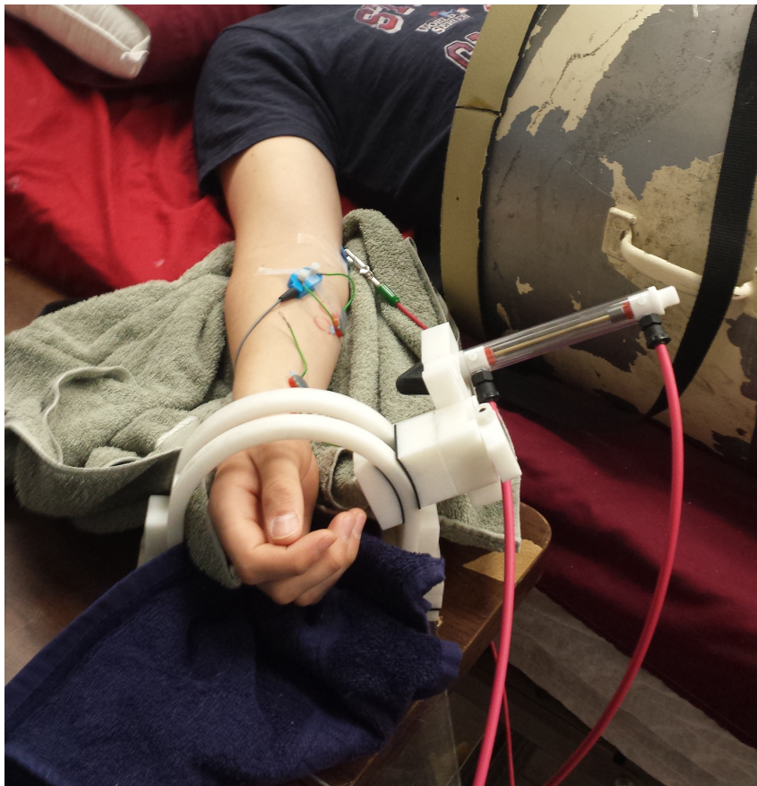
Figure 7.1: Experimental Setup with Mechanical Stimulus Device and EMG Electrodes
