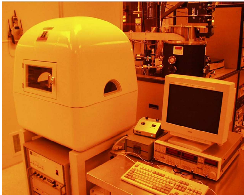
Figure 102: Hysitron nano indentation system owned and maintained at Georgia Tech IEN.
