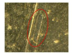
Figure 4.2 Bubble in sample channel.
