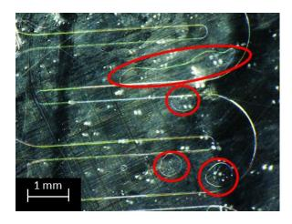
Figure 2.3 Bubble formations in sample channel.
