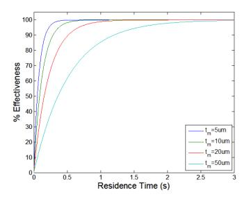
Figure 2.6 Device performance with different membrane thicknesses.
