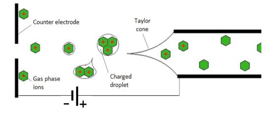
Figure 1.1 Electrospray Ionization process.
