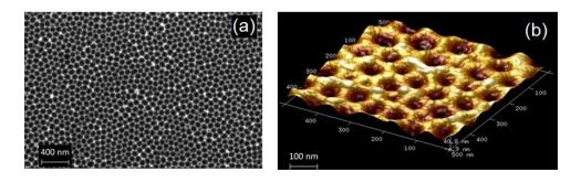
Figure 3.5 (a) SEM micrograph and (b) AFM tapping mode scan of alumina membrane.
