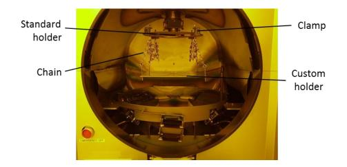
Figure 3.3 E-beam evaporation chamber during deposition of alumina precursor material.
