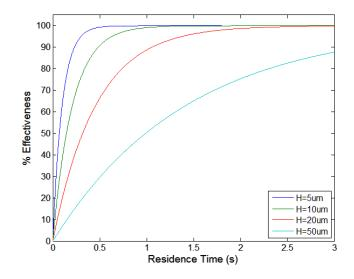
Figure 2.4 Device performance with different sample channel heights.
