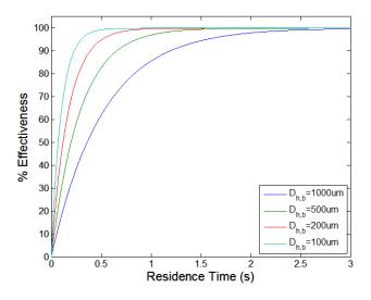
Figure 2.5 Device performance with different buffer channel hydraulic diameters.
