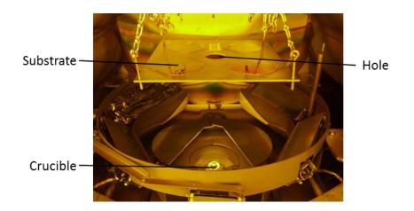
Figure 3.4 Custom substrate holder during deposition of alumina precursor material.
