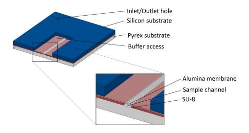
Figure 3.1 Cross sectional view of microdialysis device (not to scale).
