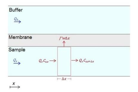
Figure 2.1 Differential element of sample flowing in microdialysis device.
