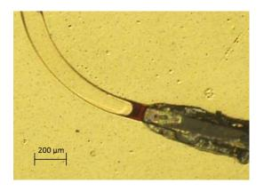
Figure 3.7 SPR 220 Photoresist clog in sample channel.
