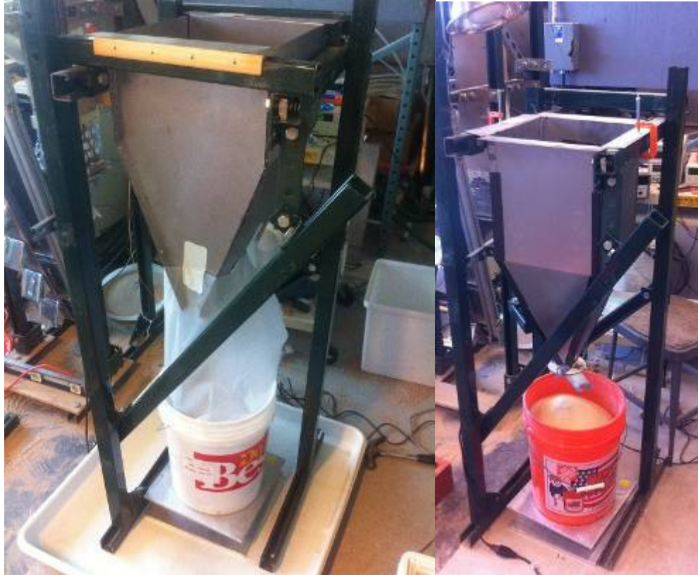
Figure 20 – Lab scale hoppers used in flow testing. Left – quasi-3D wedge hopper. Right – 3 dimensional tetragonal hopper.
