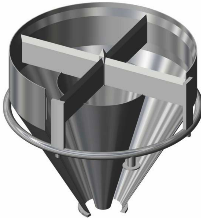
Figure 43 - BINSERT ® hopper insert system used to convert a funnel flow hopper to a mass flow hopper. Material flows both through and around the small interior cone. From Jenike.com (2013).
