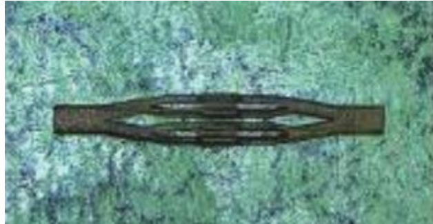
Figure 2.9 Image of single crystal SiC heat sink with tree-branch structure. [51]
