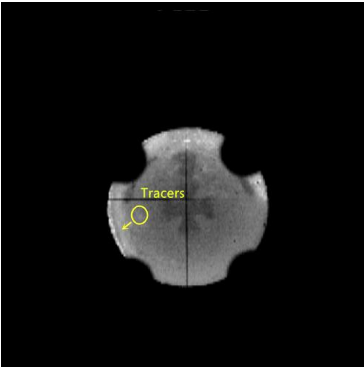
Figure 2.2: Laminar flow—tracer particles (white part in the circle) move closer to the equator.
