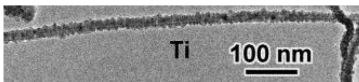
Figure 2.3 Single-wall CNT coated with titanium by chemical vapor deposition
