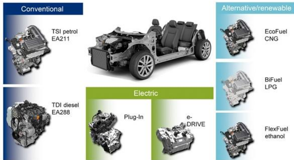
Figure 2-1: Volkswagen's new Modular Transverse Matrix drive systems ( http://www.volkswagenag.com )
