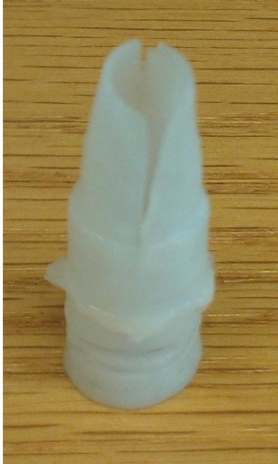
Figure 62: Valve after undergoing 500,000 cycles at 6 Hz.
