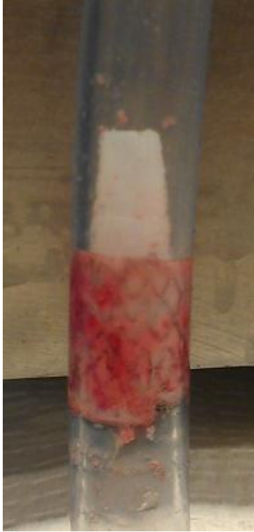
Figure 73: Outside view of valve after being in the blood flow loop for three hours.
