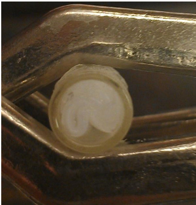
Figure 74: 10mm valve placed in 16 Fr (5.3 mm) inner diameter tube.
