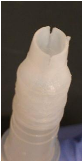
Figure 63: Valve before (left) and after (right) undergoing 500,000 cycles at 3 Hz.
