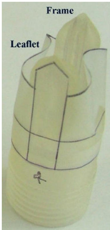
Figure 31: Second generation prosthetic valve developed by researchers from the University of Akron (image from [138]).
