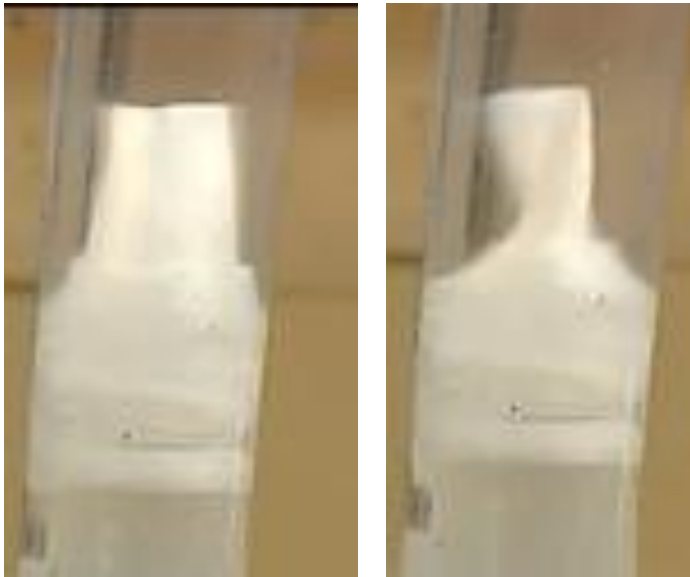
Figure 64: Example of Frames used to determine valve closure time. Frame 0 (Left). Frame 2 (Right).
