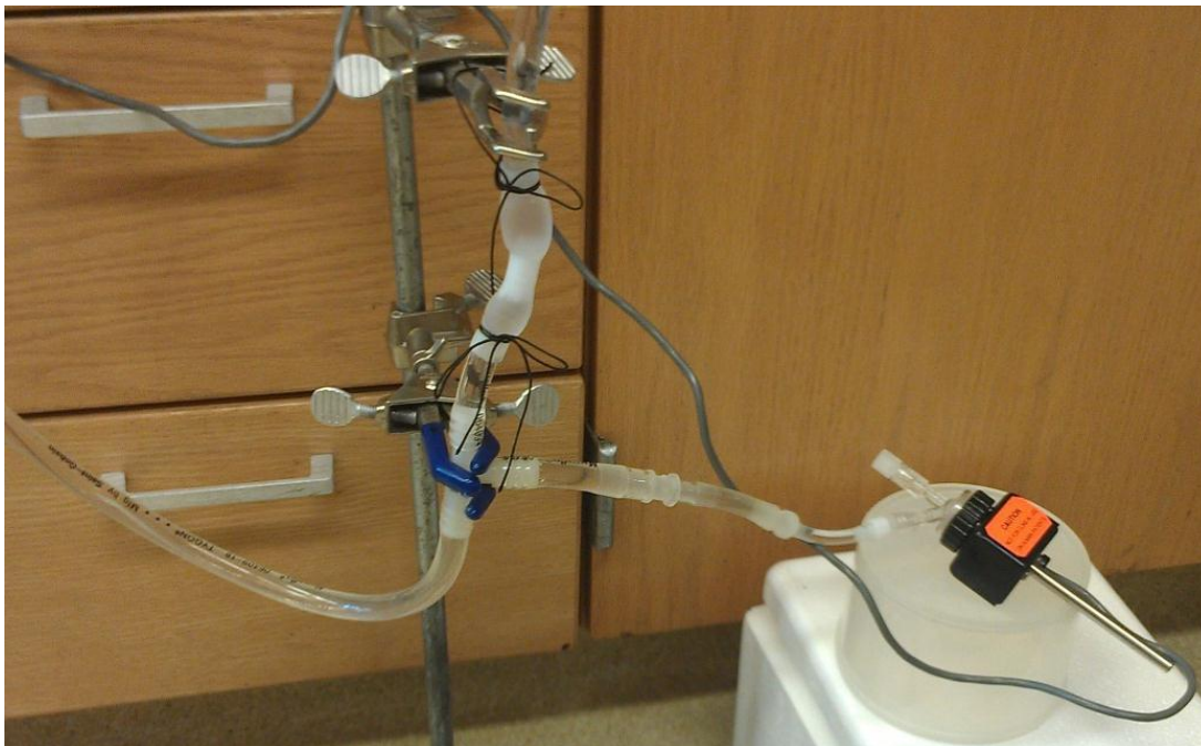
Figure 65: View of valve and pressure transducer in the distal pressure rise test.
