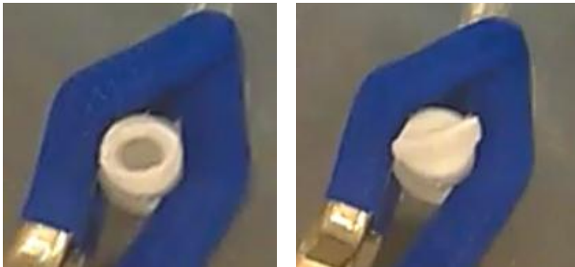
Figure 42: Proximal views of the prototype valve when open (left) and closed (right).
