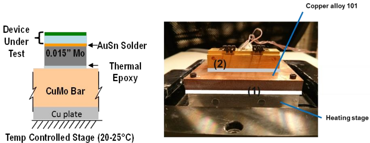
Figure 37: (Left) Schematic of GaN on SiC / GaN on Diamond device [62] (Right) Experimental set-up: Thermal grease (Silicone-based zinc oxide filled polysiloxane) was applied in (1), between the heating stage and the copper mount, Silver-based thermal compound was applied in (2), between the copper mount and the package, where the thermal conductivity of it is 6 W/m-K. Also, bolts were screwed between the package and the copper mount, and between the copper and the heating stage to immobilize the device during the micro-Raman process
