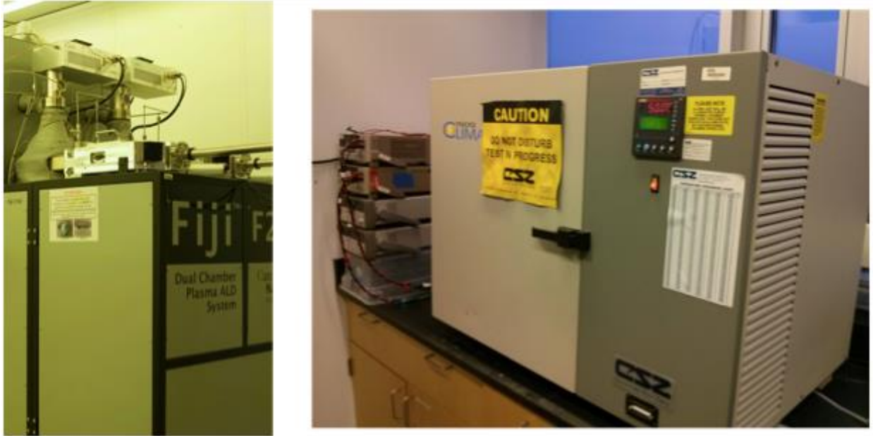
Figure 61: Cambridge Fiji Plasma ALD system (Left), Cincinnati Subzero Micro Climate Humidity Chamber at 50 °C and 85 % RH (Right)
