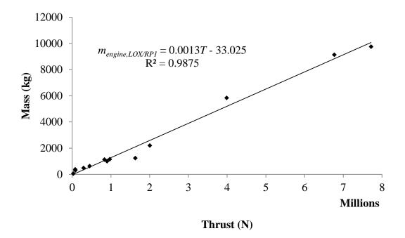
Figure A 7: Mass of a LOX/RP1 engine as a function of engine thrust
