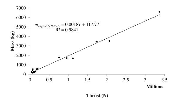
Figure A 6: Mass of a LOX/LH2 engine as a function of engine thrust
