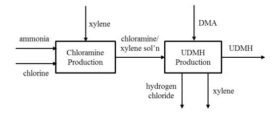
Figure 15: Representation of UDMH production
