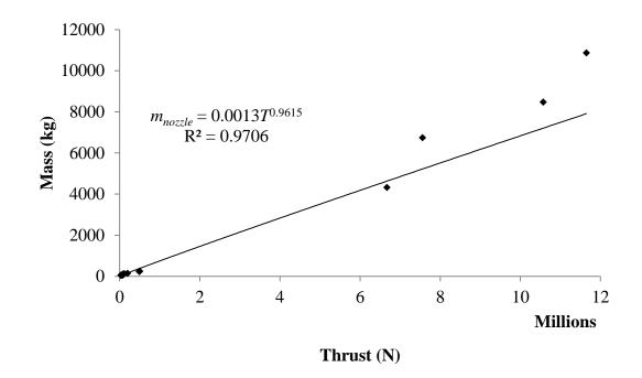
Figure A 4: Solid motor nozzle mass as a function of motor thrust
