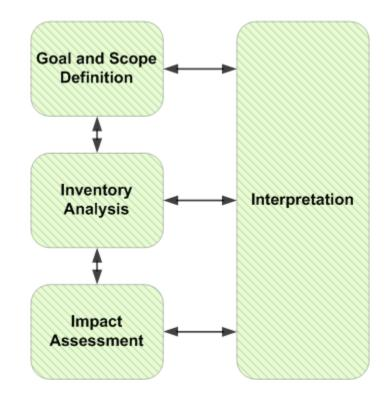
Figure 9: Parts of an LCA according to ISO 14040 and 14044
