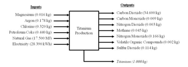
Figure 29: Production of 1 kg of titanium using Kroll Process
