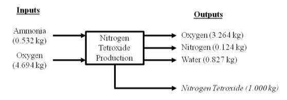
Figure 19: Life cycle inventory for the production of 1 kg of N2O4
