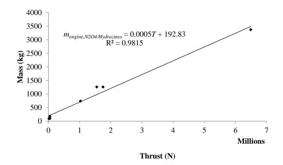
Figure A 8: Mass of an N2O4/UDMH engine as a function of engine thrust
