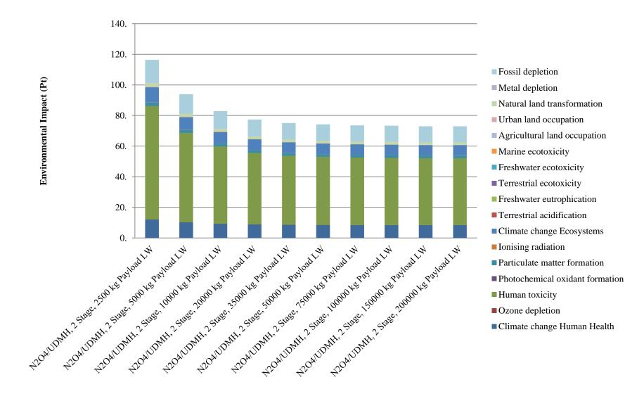
Figure D 10: Comparison of environmental impacts across lift capacities for the light-weighted two stage, N2O4/UDMH rockets, normalized for 1 kg payload to LEO, using the ReCiPe 2008 Egalitarian Endpoint single score indicator
