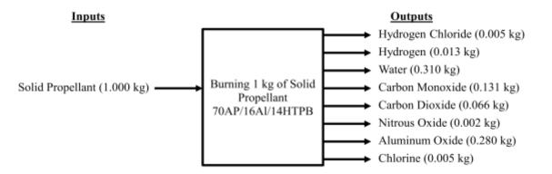
Figure 25: Mass flows associated with burning 1 kg of a solid propellant made up of 70% AP, 16% Al, 14% HTPB
