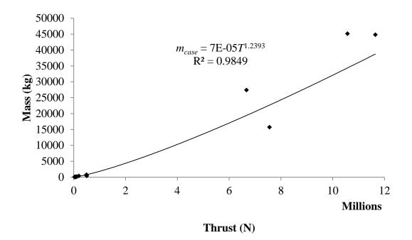
Figure A 2: Solid motor case mass as a function of motor thrust
