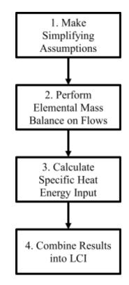
Figure 34: Graphical representation of calculation procedure in the Carbon Fiber Production Model
