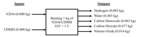
Figure 24: Mass flows associated with burning 1 kg of a N2O4/UDMH propellant mixture with an O/F ratio of 1.5
