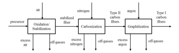
Figure 32: Representation of carbon fiber production
