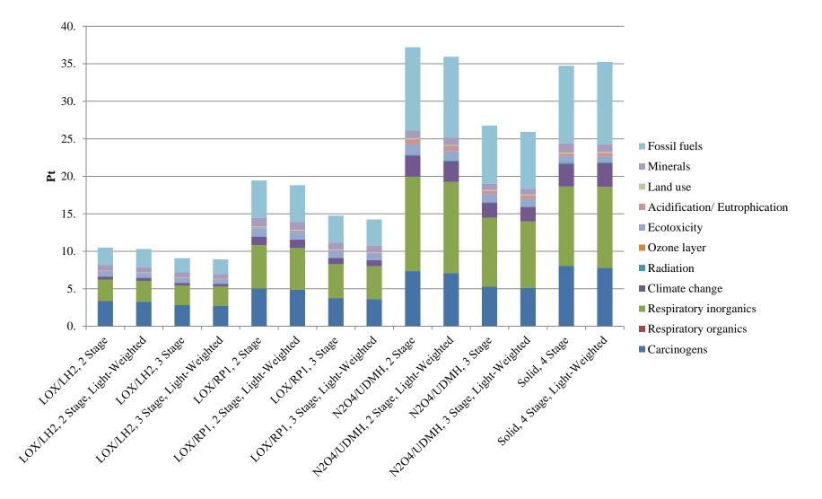
Figure 56: Life cycle impact assessment results for launching 1 kg to LEO, using Eco-indicator 99 methodology
