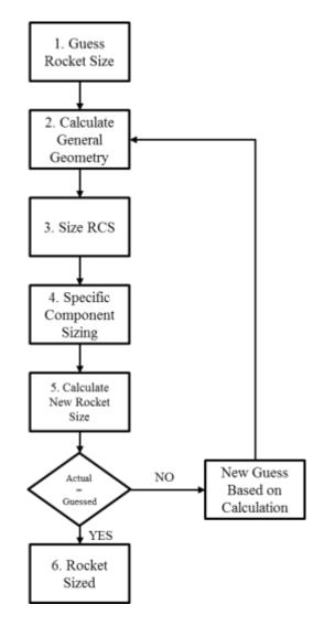
Figure 12: Graphical representation of rocket sizing procedure
