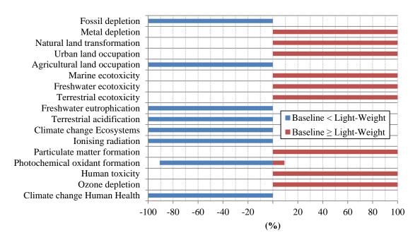
Figure E 2: Categories for which light-weighting was an improvement during the low uncertainty analysis, and the likelihood of this occurrence for the two stage, 10,000 kg to LEO, LOX/LH2 rocket, using the ReCiPe 2008 Egalitarian Endpoint single score indicator
