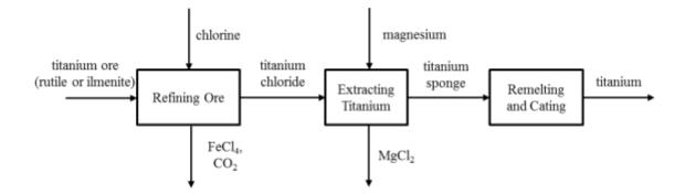
Figure 28: Graphical representation of titanium production
