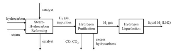
Figure 13: Representation of liquid hydrogen production process
