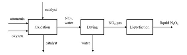
Figure 18: Representation of nitrogen tetroxide production
