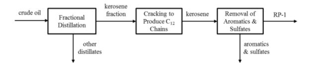
Figure 14: Representation of RP-1 production
