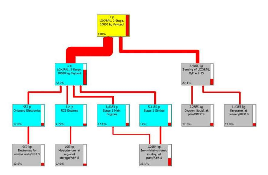
Figure 44: SimaPro LCA results using the ReCiPe 2008 Egalitarian Endpoint single score impact for a 3 stage LOX/RP1 rocket with 10,000 kg to LEO
