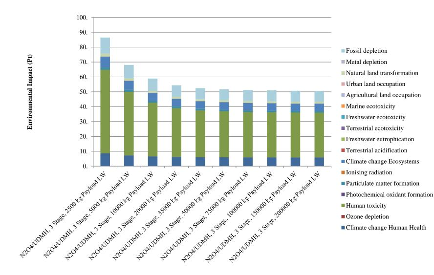
Figure D 12: Comparison of environmental impacts across lift capacities for the light-weighted three stage, N2O4/UDMH rockets, normalized for 1 kg payload to LEO, using the ReCiPe 2008 Egalitarian Endpoint single score indicator
