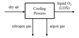
Figure 17: Representation of liquid oxygen production
