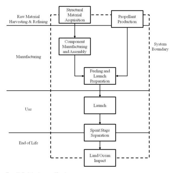
Figure 10: Typical rocket system life cycle stages
