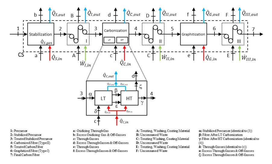
Figure 33: Graphical representation of the carbon fiber production process under consideration with the carbonization sub-processes defined
