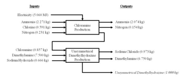
Figure 16: Production of 1 kg of unsymmetrical dimethylhydrazine
