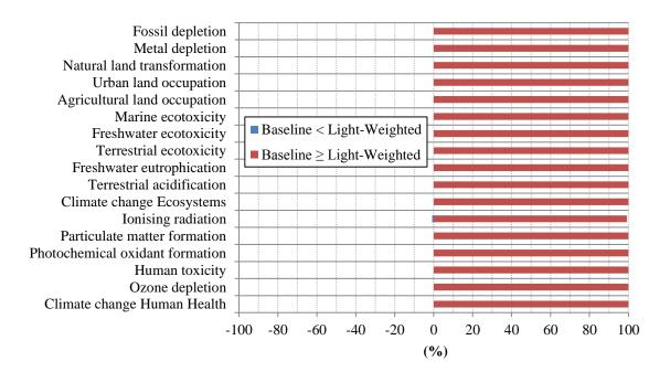
Figure E 40: Categories for which light-weighting was an improvement during the high uncertainty analysis, and the likelihood of this occurrence for the thre stage, 10,000 kg to LEO, N2O4/UDMH rocket, using the ReCiPe 2008 Egalitarian Endpoint single score indicator
