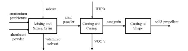
Figure 20: Graphical representation of solid propellant preparation
