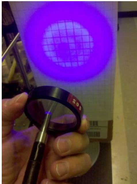
Figure 26 Photograph showing the intensity profile resulting from the UV light source from the light guide
