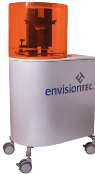
Figure 5 Photograph of EnvisionTec's Perfactory Machine [11]
