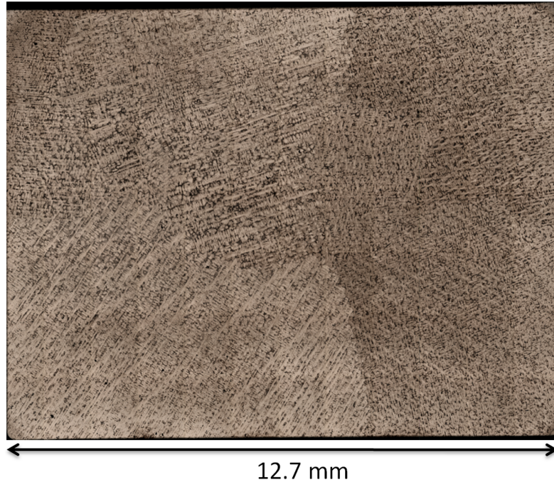
Figure 1.1: Example grain size – scale: 12.7 mm width. Optical microscopy image of microstructure exposed with Kalling’s Etchant No. 1.
