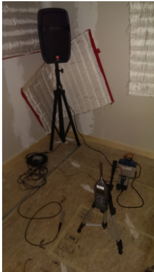
Figure 4.15: Equipment used for RT60 measurements of test house interior
