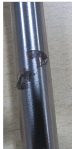
Fig 5.3 Fretted 10K_A specimen after 10K cycles of fretting
