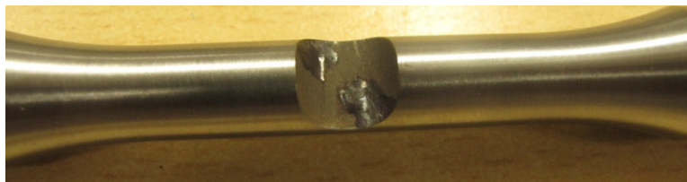
Fig 5.3 Fretted 10K_A specimen after 10K cycles of fretting
