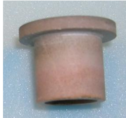
Figure 33. Ceramic sleeve used to shield the thermocouples and insulation from the flame
