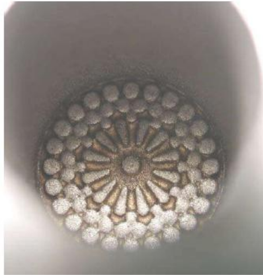
Figure 18. Failed pin array structure in WL10 after EDM [44]
