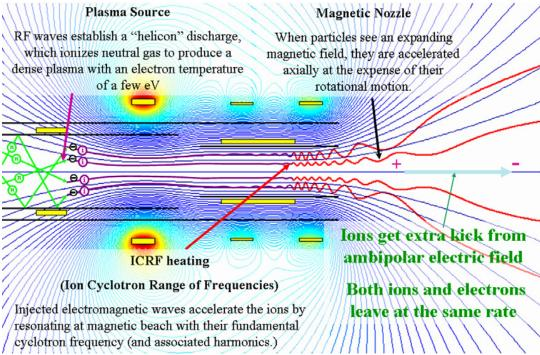
Figure 2.3. VASIMR Linear Accelerator (Bering 2008)
