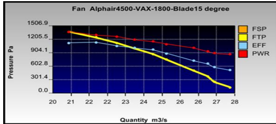
Figure 4.4. Alphair 4500-VAX-1800-Blade 15 degree
