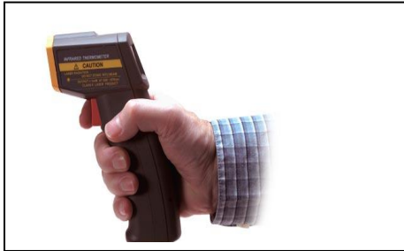
Figure 3.1 Hand-held infrared thermometer (Series Super Low Cost Infrared Thermometer)
