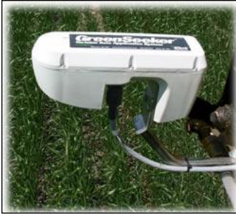
Figure 3.2 Green Seeker Optical sensor unit.
