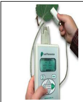
Figure 3.3 Lightweight menu-driven Leaf Porometer.
