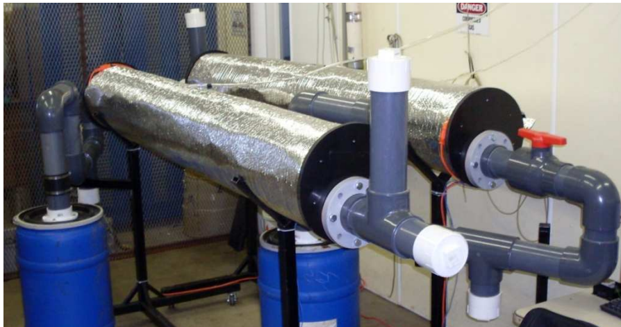
Figure 7. Photo of Sub Pilot-Scale Anaerobic Digesters.
