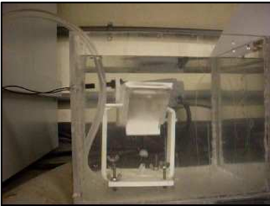
Figure 18. Photo of inverted, calibrated tipping-bucket gas meter submerged in water.
