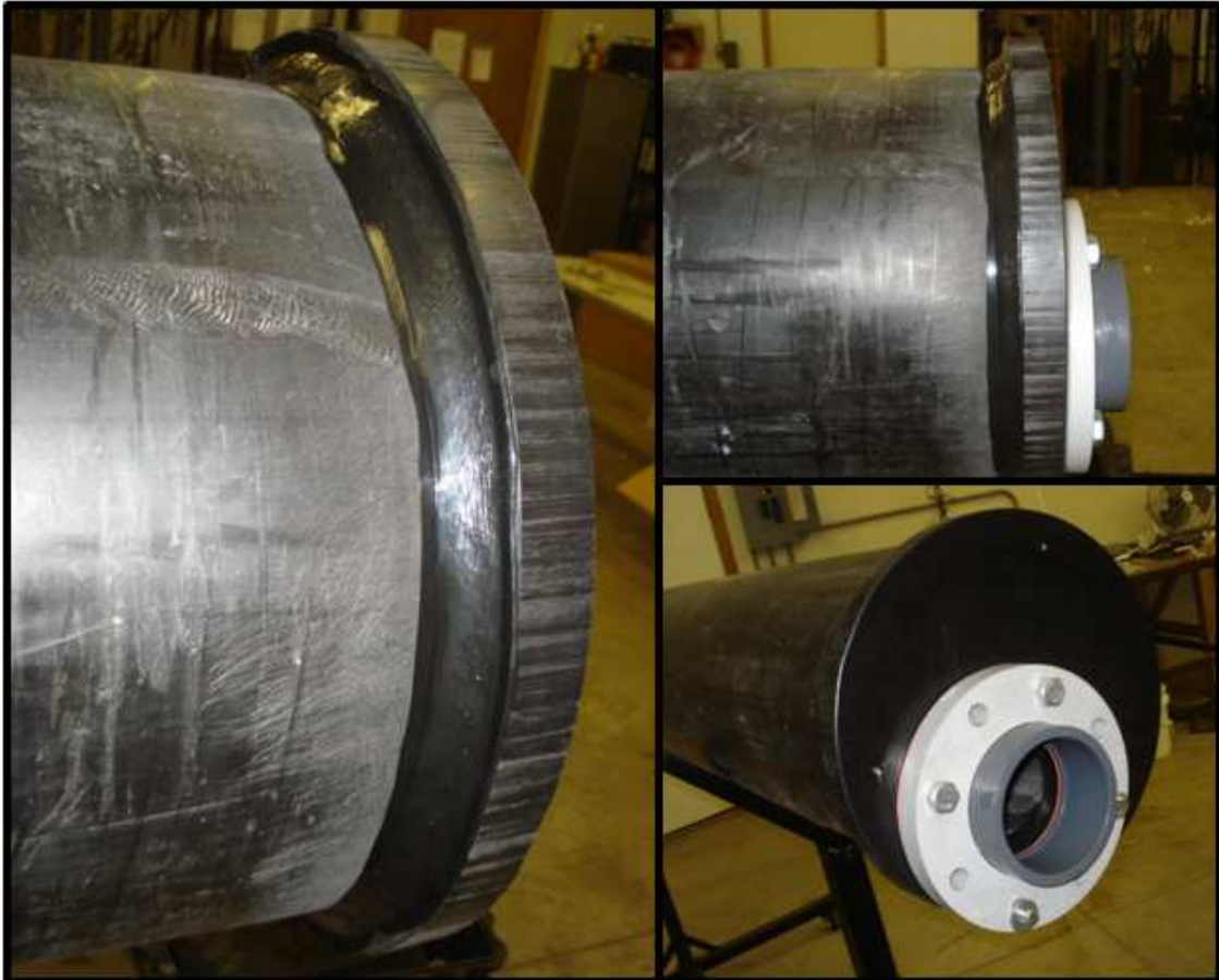
Figure 14. Photos depicting digestion tube end caps.
