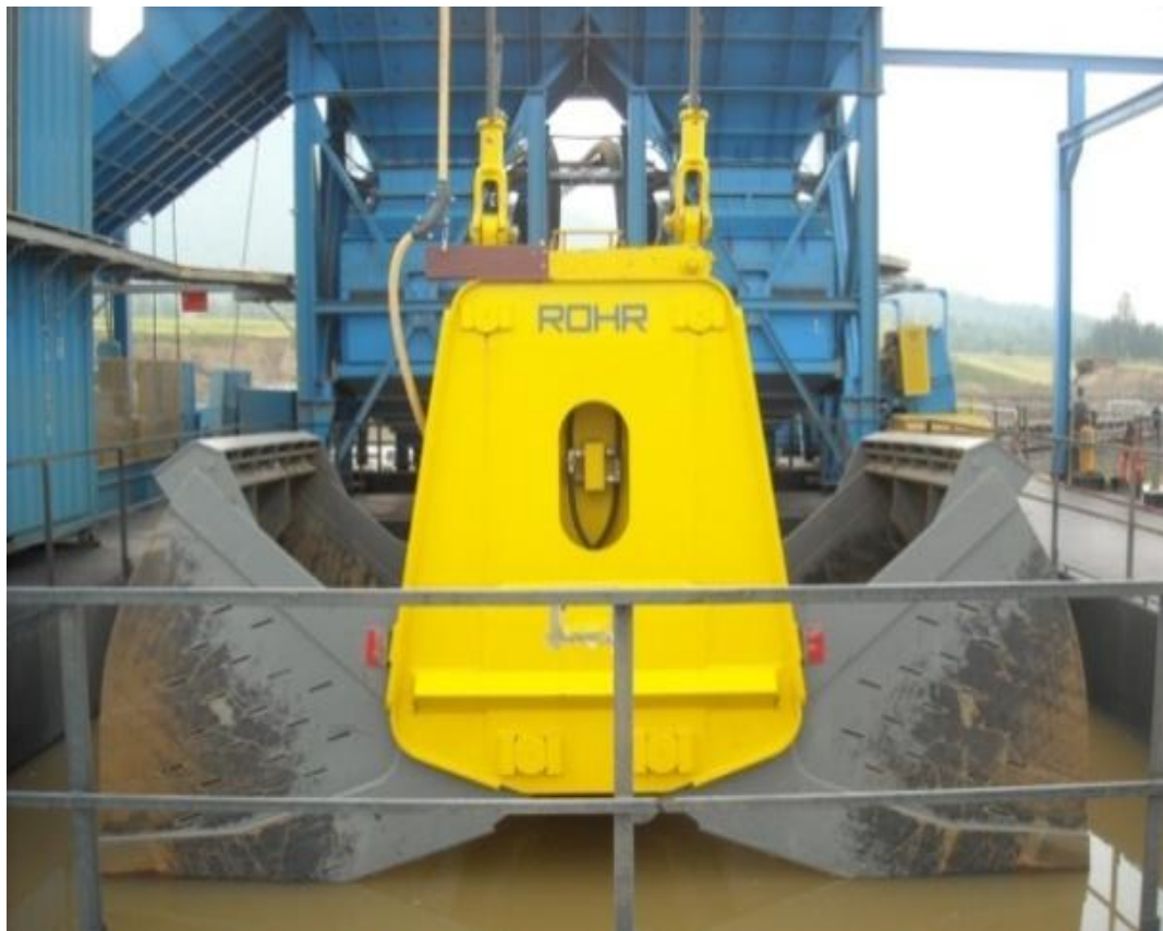
Figure 3.2 A Clamshell dredge being lowered under water
