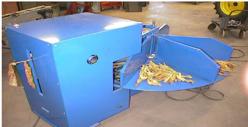
Figure 2.10: Semi-automated stripping and sorting machine.
