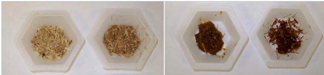
Figure 6.5. (From left to right) Raw corn stover, NaOH-pretreated corn stover, and solid fractions following enzymatic hydrolysis performed at 5% and 20% (w/w) solids and [E] = 60 FPU/g solids.
