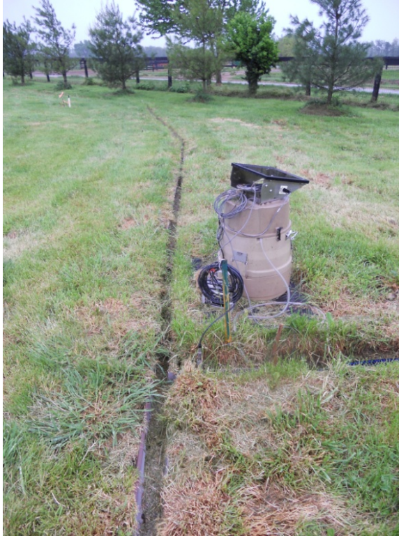
Figure 3.11: Guttering System Used to Direct VFS Runoff to Central Monitoring Point.
