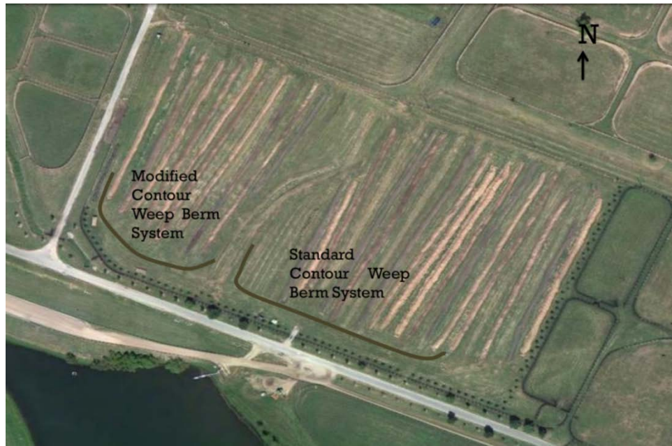
Figure 3.3: Aerial Photo of Horse Muck Composting Facility with Contour Weep Berm Locations. Source: Google Earth.
