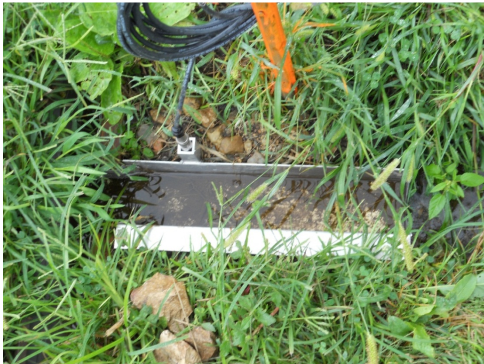
Figure 3.12: Weir and Stilling Well Used in Monitoring VFS Runoff.
