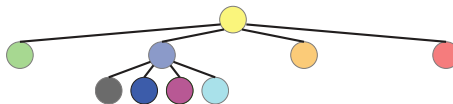
(f) Four children nodes, each correspond to a child quadrant of matching color, branch off from the navy-blue node, which is the graph representation of the quadrant that is subdivided.
