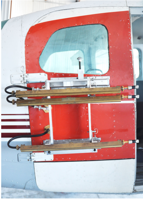
Figure 3.6: TIMMi Ka-band antennas mounted on a Cessna 206 cargo door. The top two slotted waveguide antennas receive, and the bottom antenna transmits.
