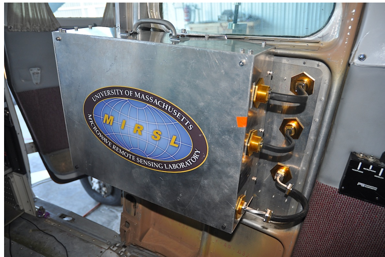
Figure 3.7: The interior of the aircraft door showing mounted transceiver and flexible WR-28 waveguides
