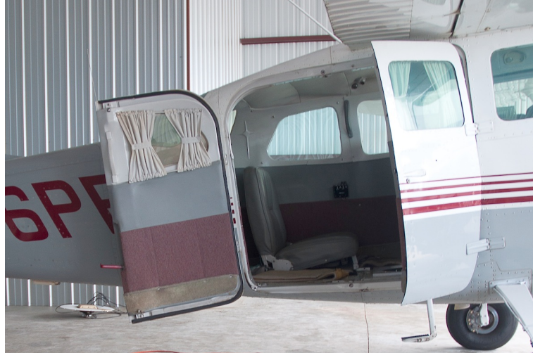
Figure 3.5: The rear cargo doors of the Cessna 206 open like a clamshell with no center pillar
