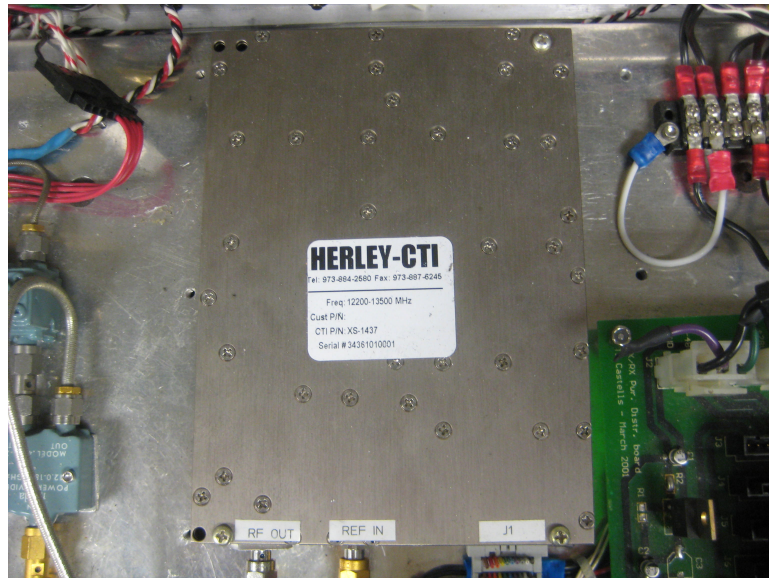
Figure 3.10: Picture of the programmable synthesizer added to the Ku-band transceiver. This new addition allows the transmitted frequency to be changed during a flight. The Herley XS-1437 has a frequency range of 12.2 GHz to 13.5 GHz.
