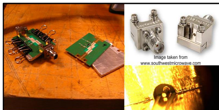
Figure B.2. A picture of the edge-coupled filters (left), the 2.4mm end-launch connectors (top-right), and the proper way to place an end-launch connector (bottom-right).
