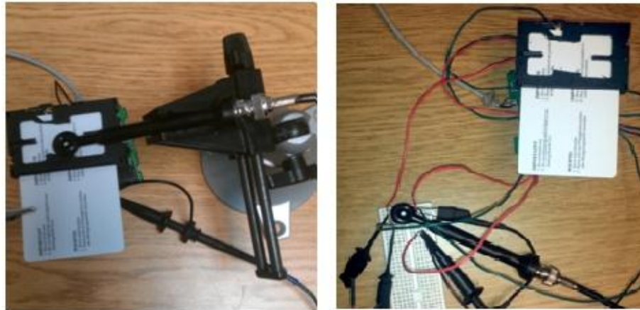
Figure 6.4 Smart card setup for Watermarking. Left side setup shows EM probe on top of the smartcard while right side setup shows EM probe near the resistor where power measurements are taken
