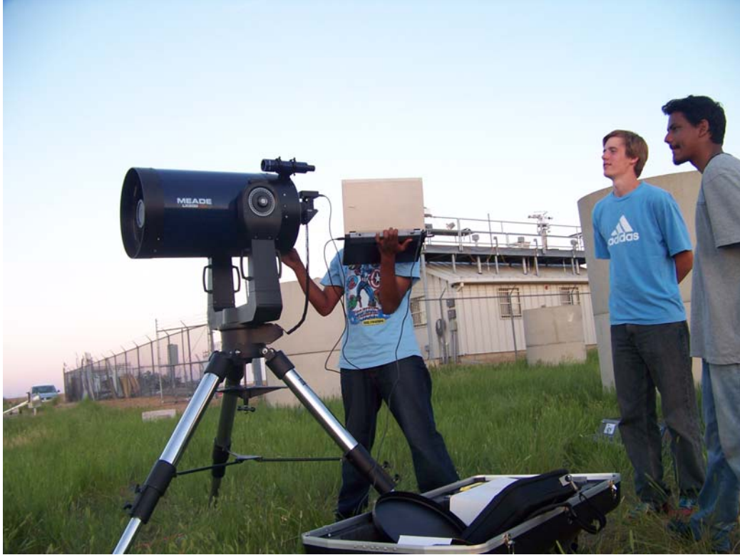
Figure 3.4. Side view of the telescope. Attached to the telescope is a CCD-camera, which collected 30 images per second. These images were saved on a laptop PC.
