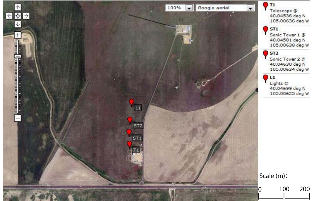
Figure 3.1. Plan view of the experimental setup at the BAO site. The 300 m high tower can be seen in the top right corner of the image. The area south-west of this tower was used to setup the entire instrumentation. The individual components are indicated by red markers, the features and locations of which are listed in the key to the top right corner of the image.
