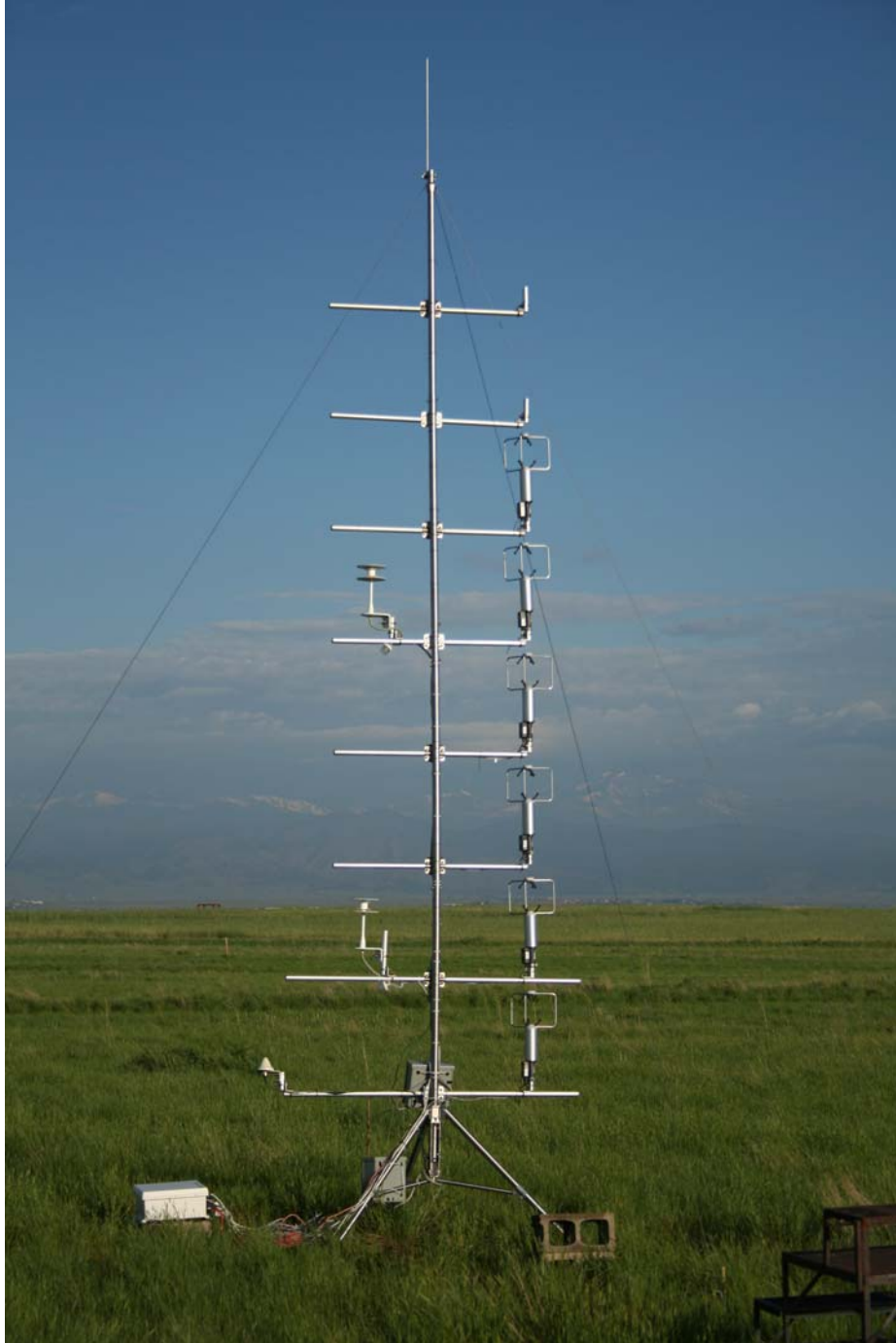
Figure 3.3. Front view of Tower 1. The central framework of the tower is a metal bar which rests on a firmly secured tripod. Crossbars mounted at various levels between 1.45 and 4.84 m AGL have sonics attached to their ends. Apart from sonics one can also see the inlets of the barometers and a GPS antenna mounted on the tower. The white box laying beside the base of the tower contains the data-logger.
