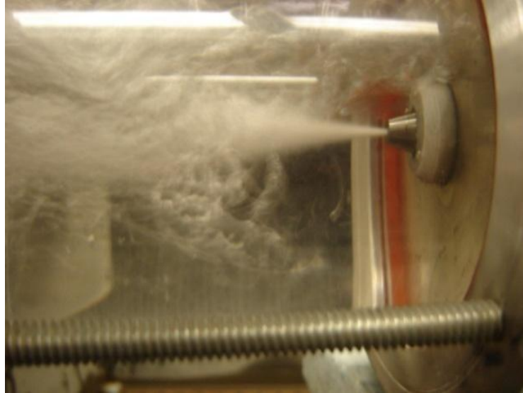
Figure 3.5. Cavitating Jet (Galecki and Mazurkiewicz, 1988)
