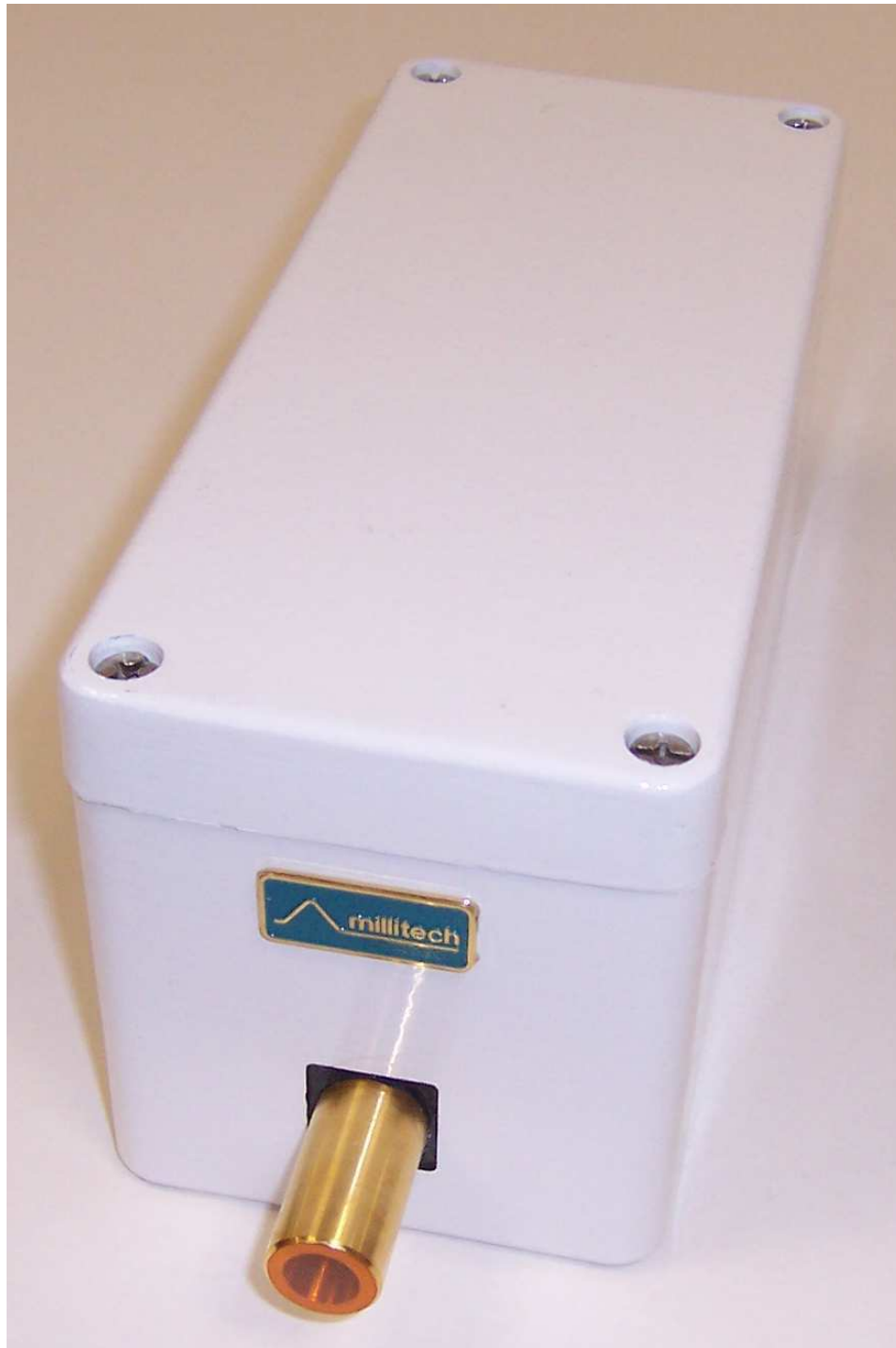
Figure C.5. 94.8 GHz Millitech noise source
