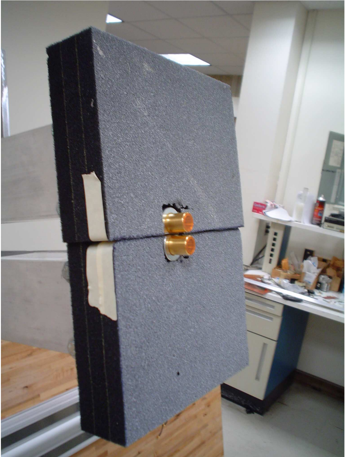
Figure C.4. 94.8 GHz Millitech radiometers on measurement structures with absorber
