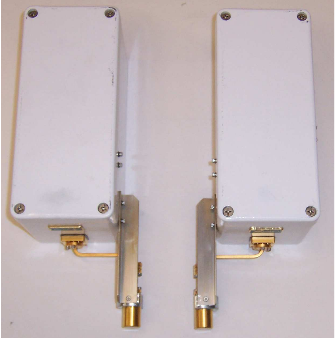
Figure C.3. 94.8 GHz Millitech radiometers
