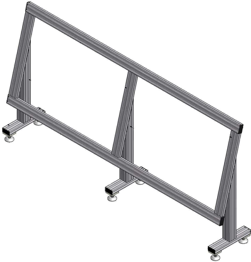
Figure 3.11. Support structure for linear drives and radiometers
