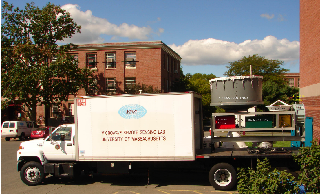
Figure 3.1: Photograph of the AMFR mobile lab, positioner, and radar subsections
